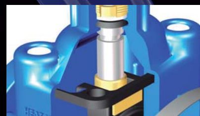
Round rubber gasket on recess in bonnet prevent blow out by pressure surges (Gate valve)
