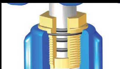
Triple O-ring stem sealing (Gate valve)
