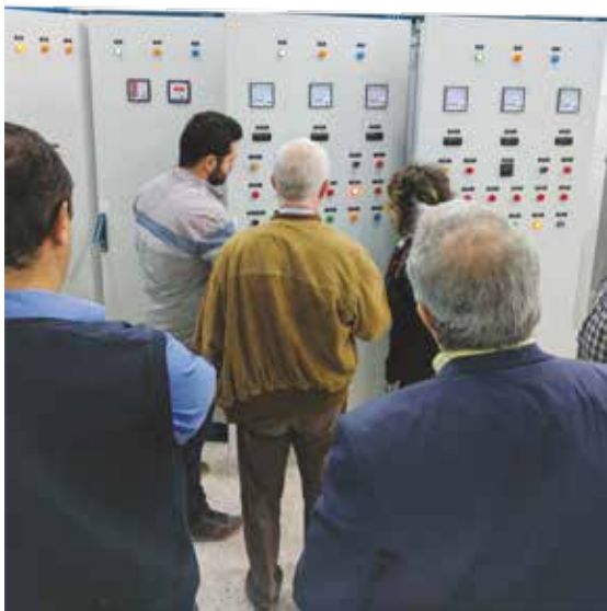
Testing of the panels in the workshop in the presence of the client/consultant
